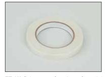
**FT-1H** fixing tape for circumferential banding of SafeTrace tracer to piping every 12" (300 mm) or as required by code or specification. Tape is 1/2" (13 mm) wide x 108' (33 m) long.
