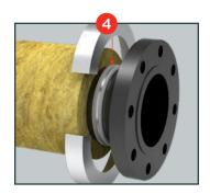
**STEP 4** Install prefabricated metal end caps into the gripping teeth and firmly lock end caps into place.
