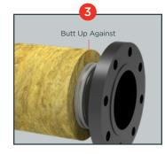
**STEP 3** Butt up insulation to the Termination Seal and install as per usual.
