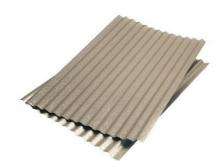
Amity Insulation's Corrugated sheets are manufactured from top grade aluminum and stainless steel with deep  $1\frac{1}{4}$  (32 mm x 6.4 mm) or  $2\frac{1}{2}$ "(64 mm x 12.7 mm) corrugations widely used to cover insulation on tanks, heat exchangers, LPG storage units, and/or food processing plants. Aluminum and stainless steel corrugated sheets are available with or without heat laminated moisture barriers.
