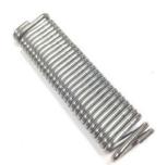
Flat (Expansion) Springs: These springs are commonly known as flat, expansion or chill springs and have a standard length of 4" (100mm) with a wire diameter of 0.12" (3mm). The maximum expansion should not exceed 2-1/2" beyond it original length. It is recommended that each spring be stretched ½" upon installation which subsequently allows 2" expansion capability per spring. Double breather springs are available when expansion requirements exceed the attributes of the standard flat 4" spring.
